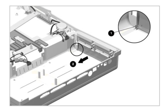
Figure 6-22. Removing the MultiBay Door
